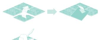
Fill any low spots, holes, chips and seams that may telegraph through the new flooring.
